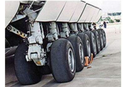
An-225 main landing gear
